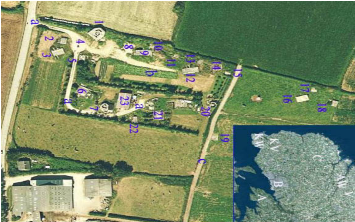
Figure 11. Stp Av 67 : general plan—(1) R 669 , (2) - (3) Vfs , (4) open emplacement, (5) Vf , (6) M 134 , (7) Flak Vf ; (8) open emplacement, (9) - (13) Vfs , (14) open emplacement, (15) - (18) Vfs , (19) possible bunker buried in the terrain, (20) Flak Vf ; (21) M 134 , (22) Vf , (23) agricultural shed; a access road, b central area, c external road; A Armorique peninsula; AW Aber Wrach; B Brest; C Cleus Foz battery; KW Keringar Wraz M.K.B. Graf Spee , KV Keringar Vihan base, V Vougo-Kerizoc radar base (Tomezzoli, 2016) [Geoportail].
